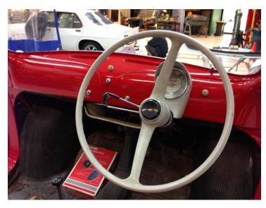
The Fiat got a full strip down and respray at the local TAFE where student panel beaters and spray painters worked enthusiastically on the Giardiniera (a vehicle they had never seen before) The Fiat needed a new front end but the other panels only needed repairs. The brakes and brake lines were once again renewed, the engine head was reconditioned as was the Carburetor. (Thanks to Parish Automotive)
